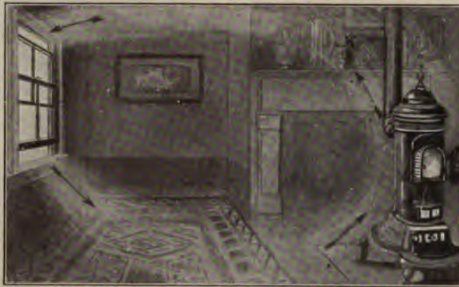
The air movements started in a room containing a heated stove and an open window. The cool air being heavier descends and flows along the floor toward the stove. Here being heated it expands, becomes lighter and rises flowing along the top of the room and out at the top of the window.
